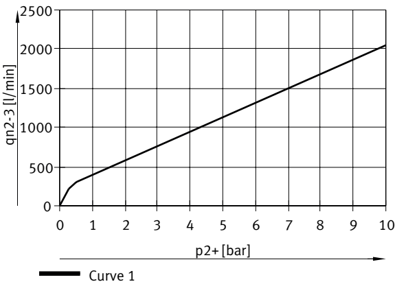
Flow rate q_n from 2 -> 3 as a function of excess output pressure p_2 , VPPM-8F/8TA-...-0L10H-... (10 bar)
